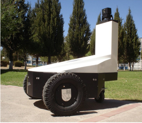
Fig. 5. Robot móvil omnidireccional IVWAN (Intelligent Vehicle With Autonomous Navigation).
