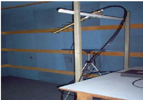
Fig. 6. Tag under test in the anechoic chamber.
