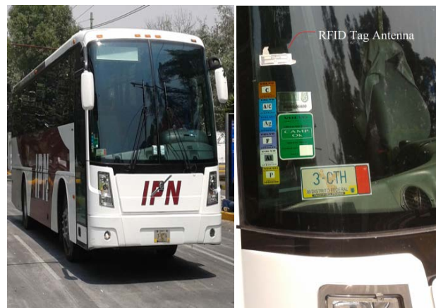
Fig. 2. RFID Tag Antenna strapped to the bus windshield.
