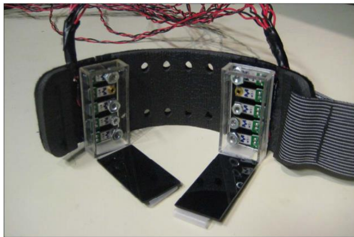
Fig. 4. Skinput Armband with 10 piezoelectric transducers [6].
