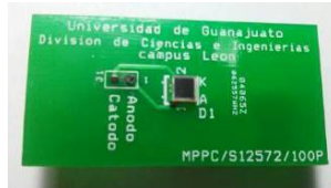
Figure 4 Photodiode board top layer.
