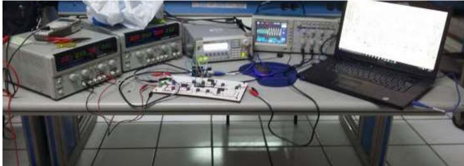
Figure 8 Photo of the measurement setup of the 64-QAM modulator.
