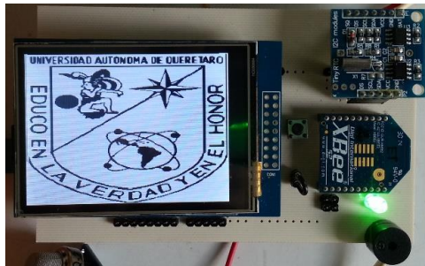
Figure 9 Signal monitoring board.
